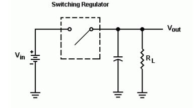
The time that the switch remains closed during each switch cycle is varied to maintain a constant output voltage. Notice that the primary filter capacitor is on the output of the regulator and not the input. As is apparent, the switching regulator is much more efficient than the linear regulator achieving efficiencies as high as 80% to 95% in some circuits. The obvious result is smaller heat sinks, less heat and smaller overall size of the power supply.
