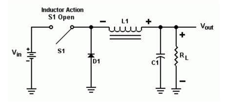
As we see in this diagram the electromagnetic field that was built up in L1 is now discharging and generating a current in the reverse polarity. As a result, D1 is now conducting and will continue until the field in L1 is diminished. This action is similar to the charging and discharging of capacitor C1. The use of this inductor/diode combination gives us even more efficiency and augments the filtering
