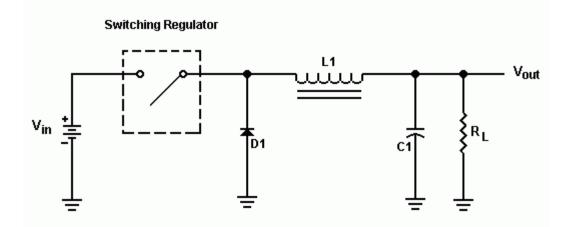
As we see above the switching regulator appears to have a few more components than a linear regulator. Diode D1 and Inductor L1 play a very specific role in this circuit and are found in almost every switching regulator. First, diode D1 has to be a Schottky or other very fast switching diode. A 1N4001 just won't switch fast enough in this circuit. Inductor L1 must be a type of core that does not saturate under high currents. Capacitor C1 is normally a low ESR (Equivalent Series Resistance) type.
