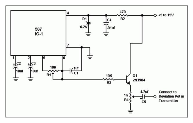
Figure 1 illustrates an easy circuit that can be constructed with mostly Radio Shack parts on any general purpose circuit board. The only rigid requirement is that capacitor C1 be stable over a wide temperature range. Use only Mylar, Polyester or Metal film for capacitor C1. The frequency is determined by the following formula:
